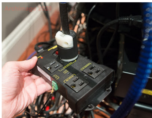
lot Relay Power Switch - trigger connected to turn on amplifier when preamp activated with remote.
